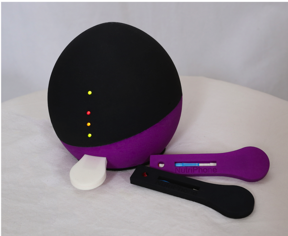
Figure 6. Tidbit, our Version 3 design and new test strip cassettes. The confusing pull-out tray has been eliminated, and the asymmetry of the device prevents users from inadvertently placing it upside down.
