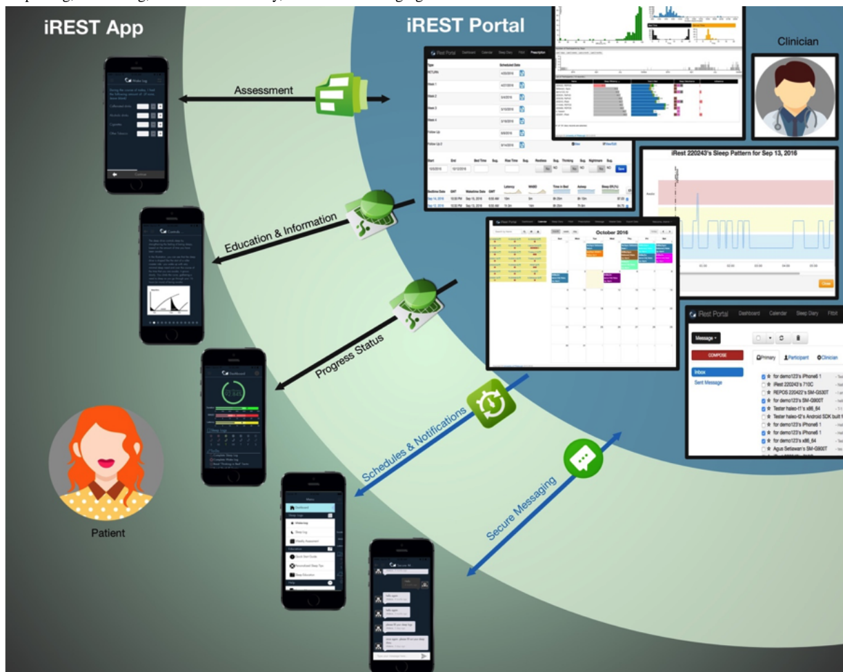
Figure 1. A model representing the iREST app and clinician-portal's two-way interactions which include: assessment, education/information delivery, progress reporting, scheduling, notification delivery, and secure messaging.
