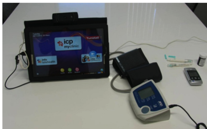
Figure 2. The in-home monitoring device of the clinical trial: a tablet PC, sphygmomanometer, and glucometer.
