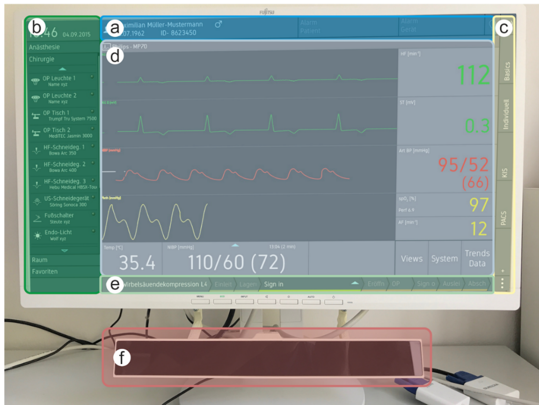
Figure 1. The anesthesia workstation (ANWS) functional model. The interface screen consists of six main elements: (a) patient context and alarms; (b) device panel: overview of all devices connected to the ANWS; (c) view mode selector; (d) area reserved for the selected view; (e) workflow process; and (f) eye-tracking system.
