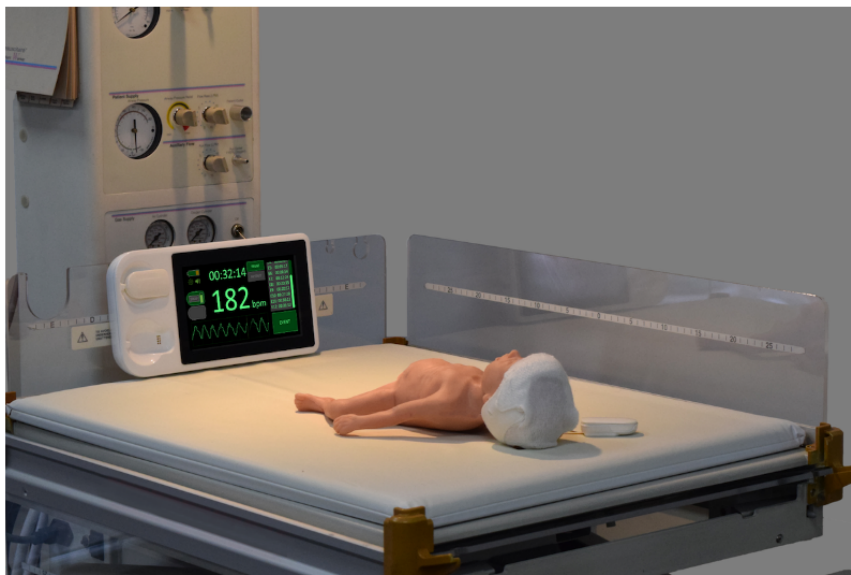
Figure 5. Resuscitation device comprises a single-use thermally insulating hat that communicates wirelessly (via battery powered modules) with a display mounted on the resuscitation table.
