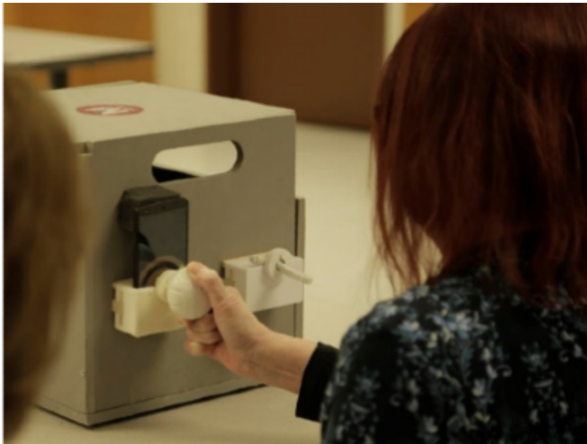
Figure 3. User turning doorknob with a smartphone in the holder and the key with a holder.
