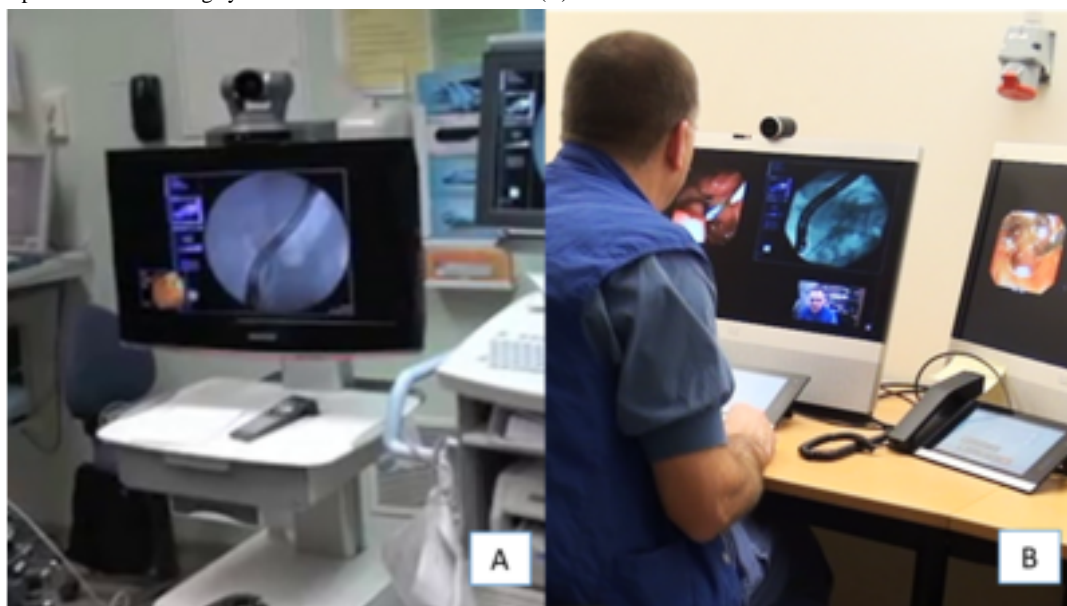
Figure 1. The remote clinics used a Polycom Realpresence Practitioner cart 8000 (A). At the central site, the consulting surgeon used a Polycom HDX4500 desktop video conferencing system with a touch screen control (B).
