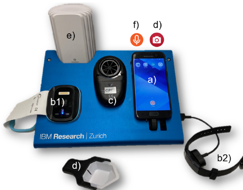
Figure 2. The CAir-Desk setup for the usability study as a collection of sensors. Items indicated here are as follows: (a) smartphone, (b1) arm-worn accelerometer, (b2) wrist-worn accelerometer, (c) spirometer, (d) sputum collector and smartphone camera, (e) environmental air quality monitor, and (f) nocturnal cough monitor.
