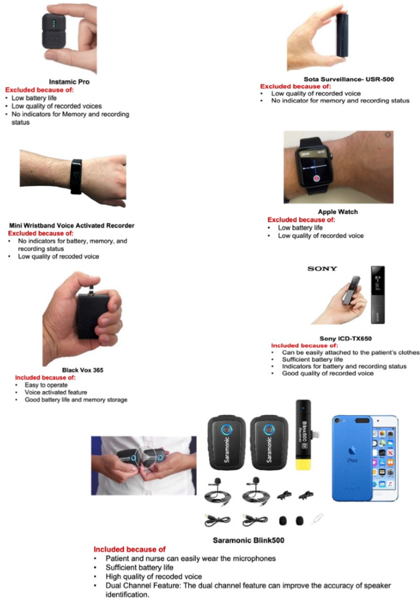
Figure 2. Audio-recording devices evaluated for audio recording of patient-nurse verbal communication.
