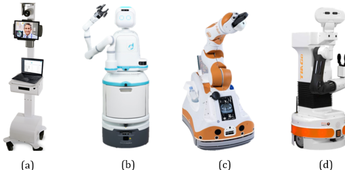
Figure 2. Representative medical robots used in hospitals during the COVID-19 pandemic. (a) Vici robot developed by InTouch Health (United States). (b) Moxi robot created by Diligent Robotics (United States). (c) Lio-A robot from F&P Robotics AG (Switzerland). (d) TIA-Go robot from PAL Robotics (Spain).
