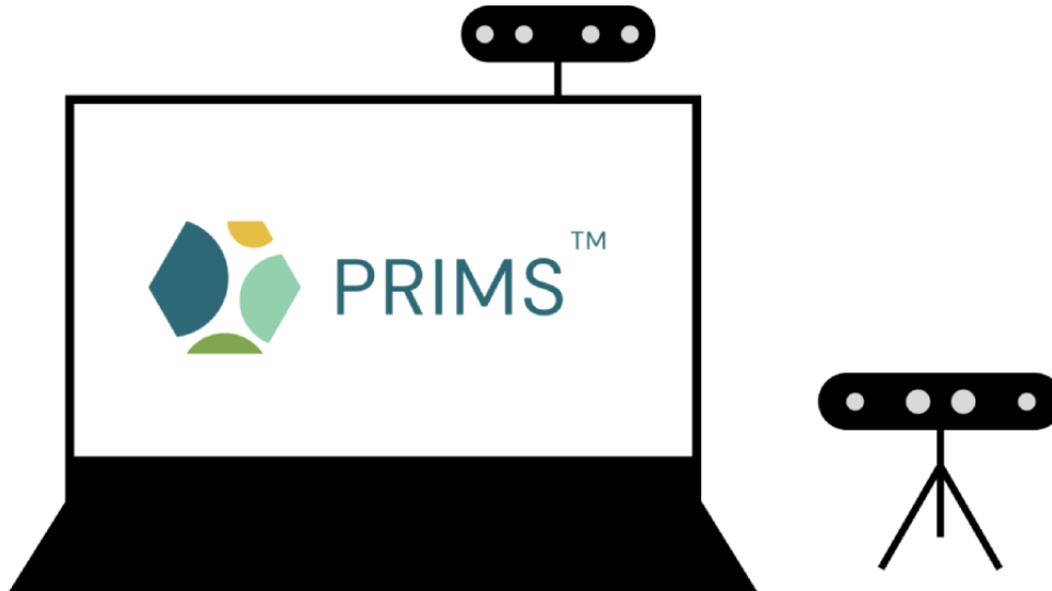
Figure 6. Diagram of hardware setup showing the position of the laptop and 2 depth cameras.
