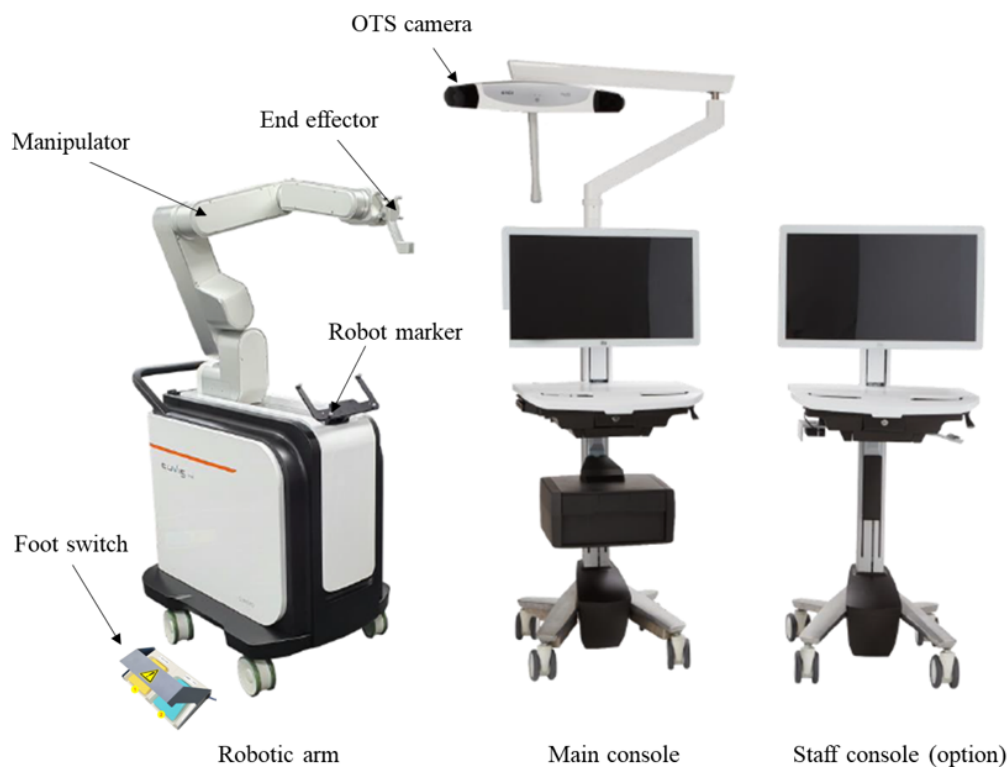
Figure 1. The CUVIS spine robot system: robotic arm (left), main console with navigation optical infrared tracking camera (middle), and the control workstation (right). OTS: optical tracking system.
