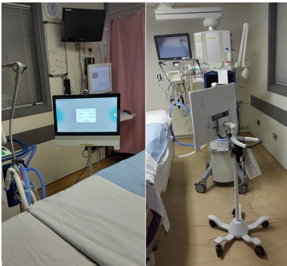
Figure 1. Video end point mounted on a mobile unit stand at an intensive care unit bedside.
