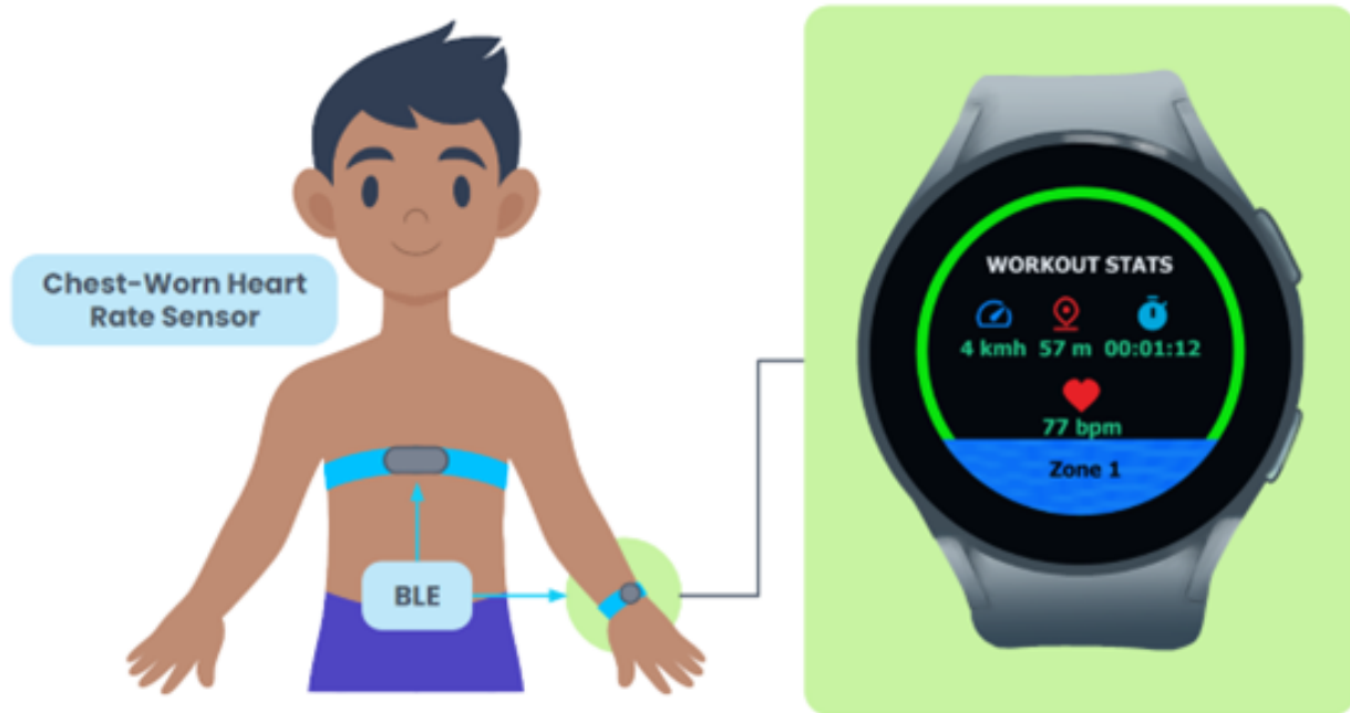
Figure 1. Smartwatch with solo workout screen connected to Bluetooth heart rate sensor. bpm: beats per minute; BLE: Bluetooth Low Energy.
