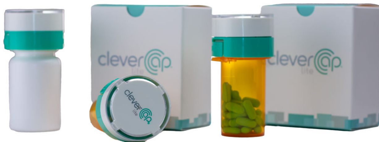
Figure 3. CleverCap device. A smart pill bottle linked with the mChoice app to track preexposure prophylaxis (PrEP) medication.
