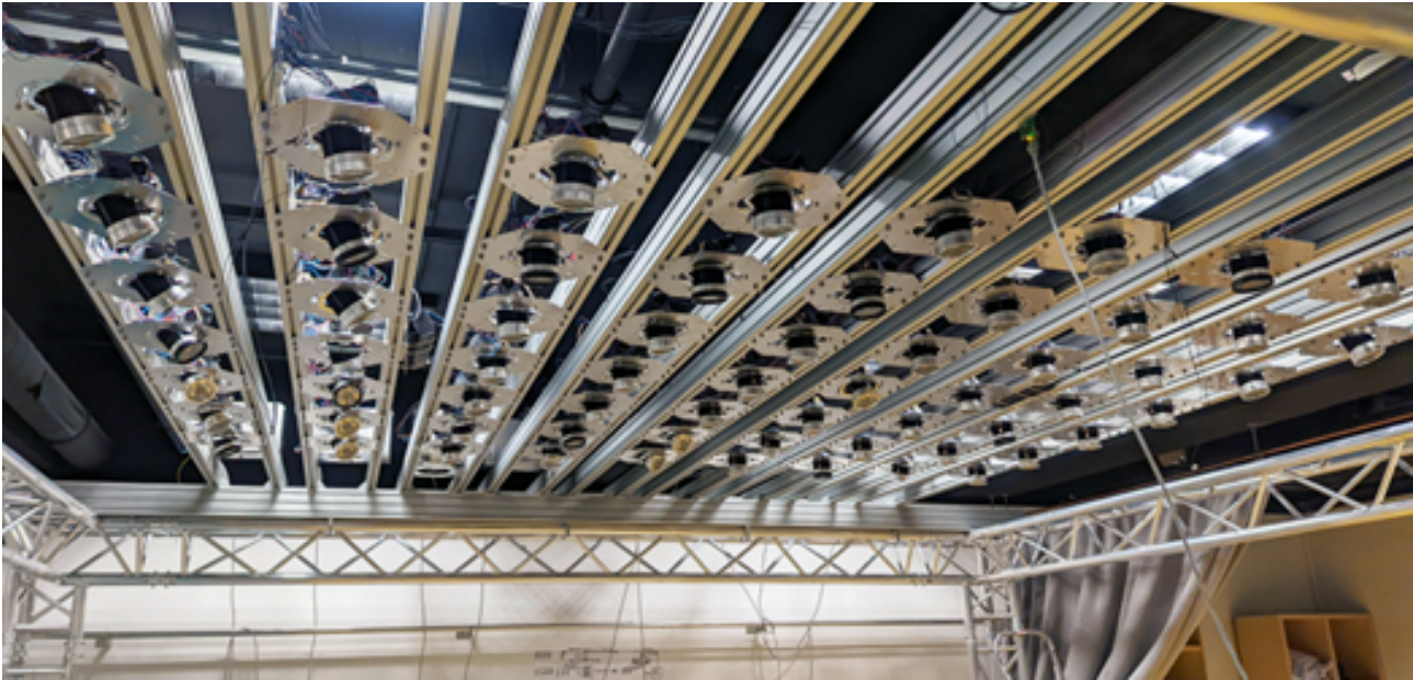
Figure 8. Smart ceiling lights used for the living laboratory study, consisting of an array of small lighting modules.
