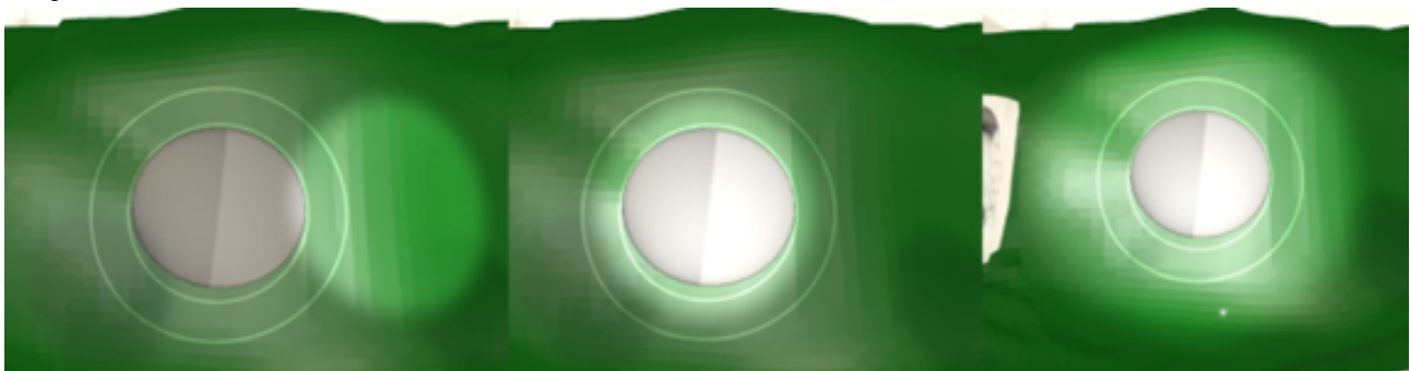
Figure 6. Examples of setting the illumination field and position of the light (left: wrong position; middle: correct setting; and right: field of illumination is too large).
