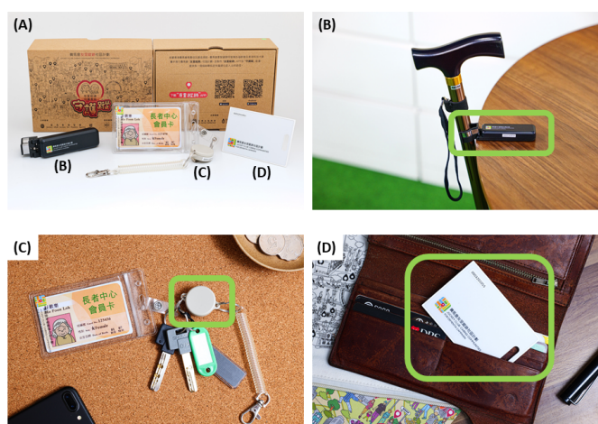
Figure 1. The Bluetooth Low Energy tag in different designs. (A) Overview, (B) walking stick holder design, (C) keychain design, and (D) smart card design.
