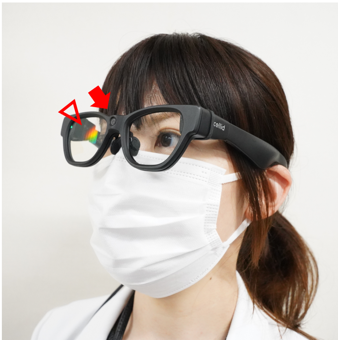
Figure 1. Photograph of a doctor wearing augmented reality glasses. A diffraction grating is installed on the right lens (framed red arrowhead), and a built-in miniature camera is located on the bridge (red arrow).
